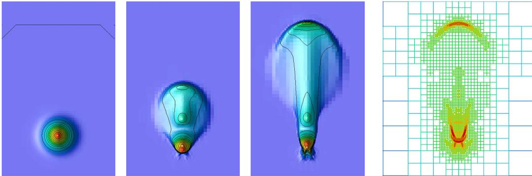
**Fig. 1** Evolution of the electron density  $n_e$  after  $t = 10$ ns, 20ns and 30ns (left). The refined grid after  $t = 30$ ns (right).
